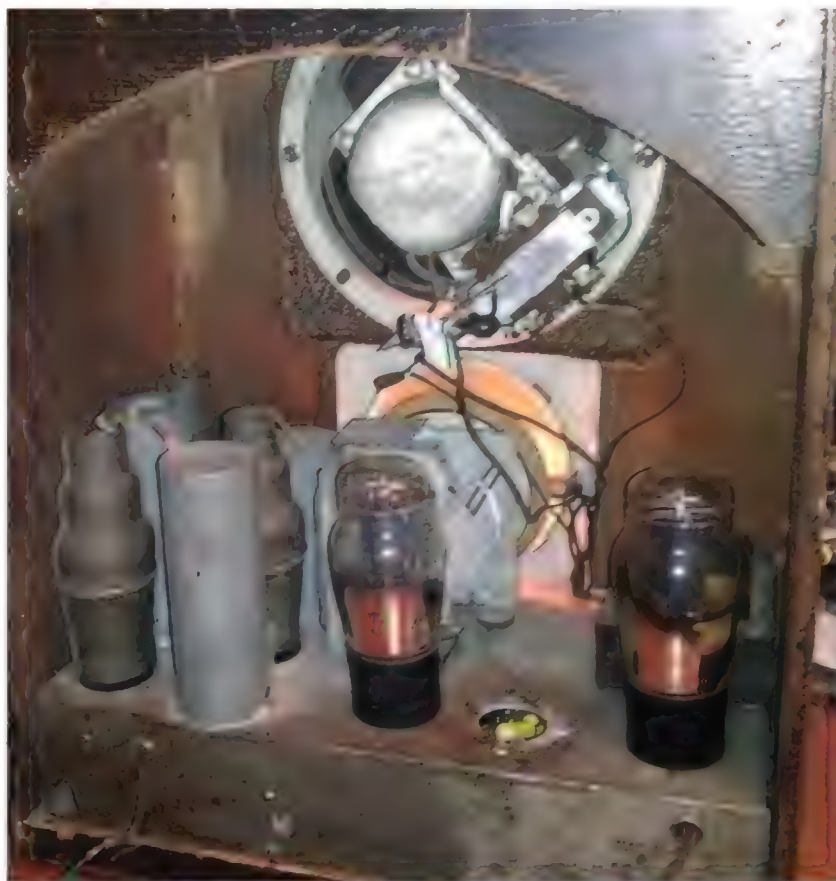
This Simplex Model P tombstone radio has an extra bolted-on output transformer, and is missing a filter capacitor can.
